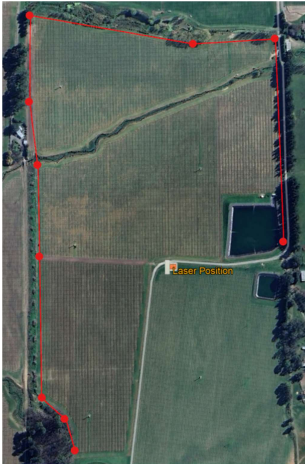
Zone 1 – Preset Sequence Mode. (Scan of high-pressure areas at dusk including roosting areas – dense trees) Speed 2, Solid Beam
