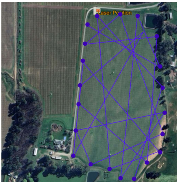
Zone 2 – Preset Random Mode (points dotted around the perimeter) Speed 4, Solid Beam
