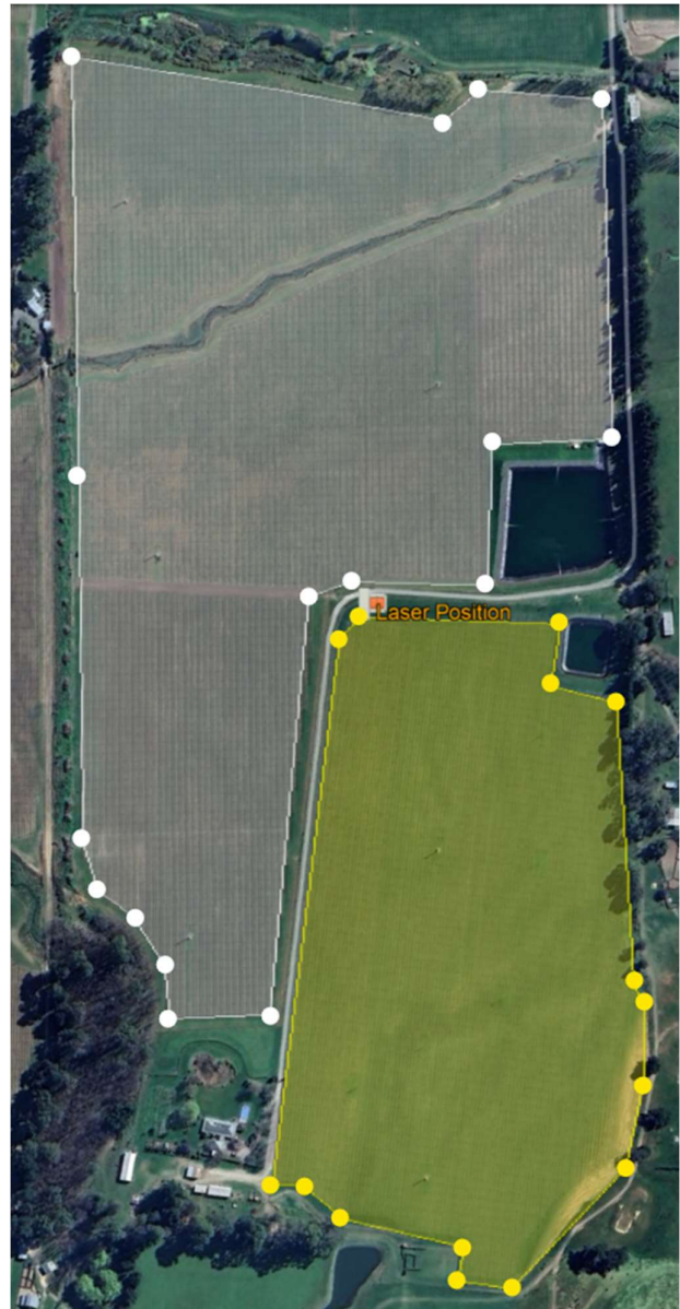
Zone 3 & 4 - Boundary Mode. Separate Zones so the beam does not cross the driveway to the house on the south. Speed 3, Fast Pulsing Beam
